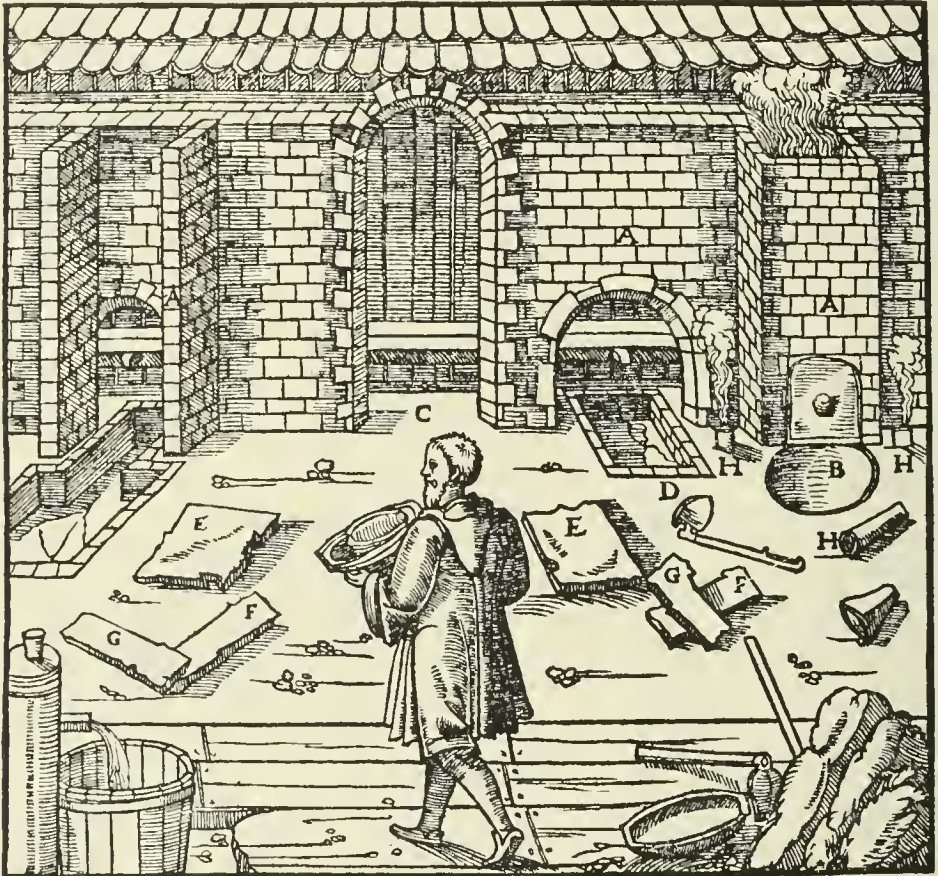
A—FURNACES. B—FOREHEARTH. C—DOOR. D—WATER TANK. E—STONE WHICH COVERS IT. F—MATERIAL OF THE VENT WALLS. G—STONE WHICH COVERS IT. H—PIPE EXHALING THE VAPOUR.
